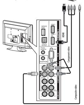
Depending on the jacks available on the cable or satellite TV box, connect a video cable from the outgoing jacks on the cable or satellite TV box to the corresponding jacks on the back of your TV. The connection can be to an HDMI jack, the COMPONENT IN/Y, PB, PR jacks, or the AV IN VIDEO (composite) jack.
